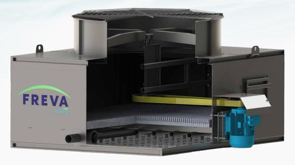
Belt driven systems are used in applications requiring lower fan speeds. It is generally used in applications with a fan diameter of 1800 mm and larger fan diameters. The system is driven by belts specially designed for the TXY series cooling tower. It provides long life with its multi-channel and high hardness. Belt drive system provides ease of maintenance. It provides low noise level on first take offs.
