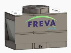
The outer body material is generally produced from sheet metal containing 600 grams of zinc per Z600 square meter. The inner and outer surfaces of the sheets are coated with polymer-based epoxy paint. Stainless steel applications are also made according to the customer's request.
